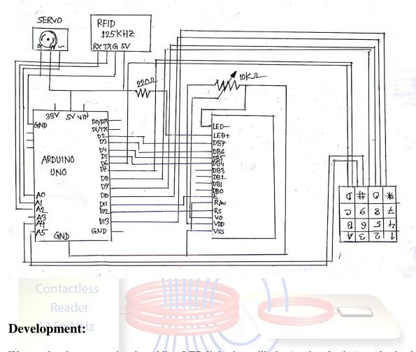
We can develop our project by adding LED light that will give us signals about authorized and unauthorized people. We can also use a clock that will show time. We also use buzzer that will make noise during unauthorized access.
