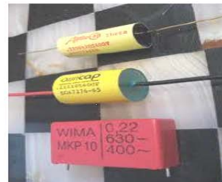
Polypropylene Film capacitor
