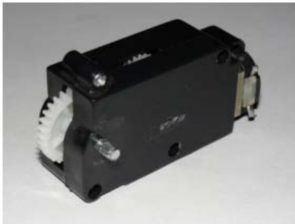
DC geared motor taken from Toy clamp
